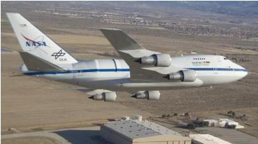
The highly modified Boeing 747SP aircraft began its first test flights in 2007 and its first science flights in 2010. In addition to the 2.5 meter (8.2 feet in diameter) telescope, the airborne observatory includes work stations for scientists and educators. According to the NASA website, over the course of its planned 20 year lifetime, "SOFIA will inspire the development of new scientific instrumentation and foster the education of young scientists and engineers."
